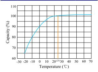
Temperature effects on capacity at 1C
